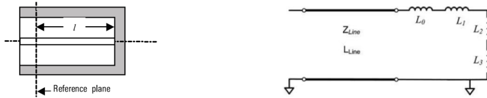
Fig 9: Internal construction and equivalent circuit diagram of the short standard
